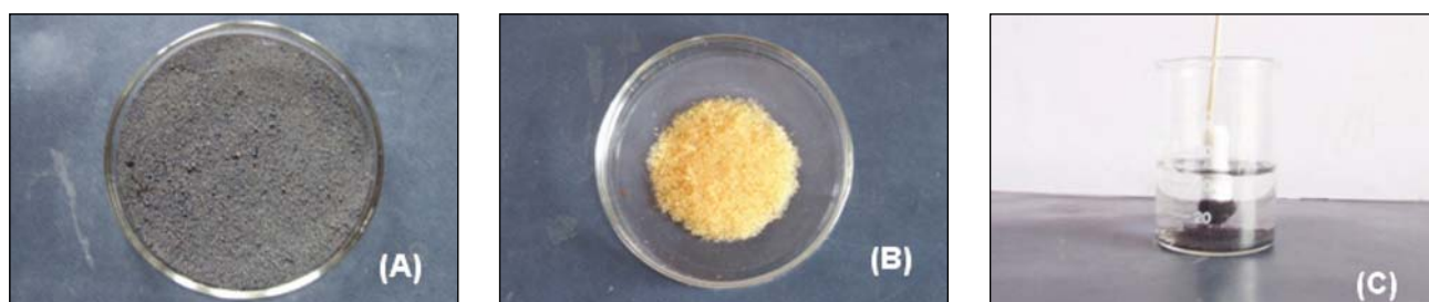
Figure 1: Photographs of (A) magnetite loaded cationic resin (MLCR), (B) plain resin and (C) their retention on the magnet surface.
